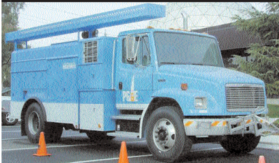
One of 29 John Deere natural gas powered Freightliner trucks developed by PG&E.
