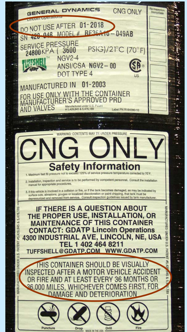
“Do not use after” and “Inspection” Warnings on CNG tank label
